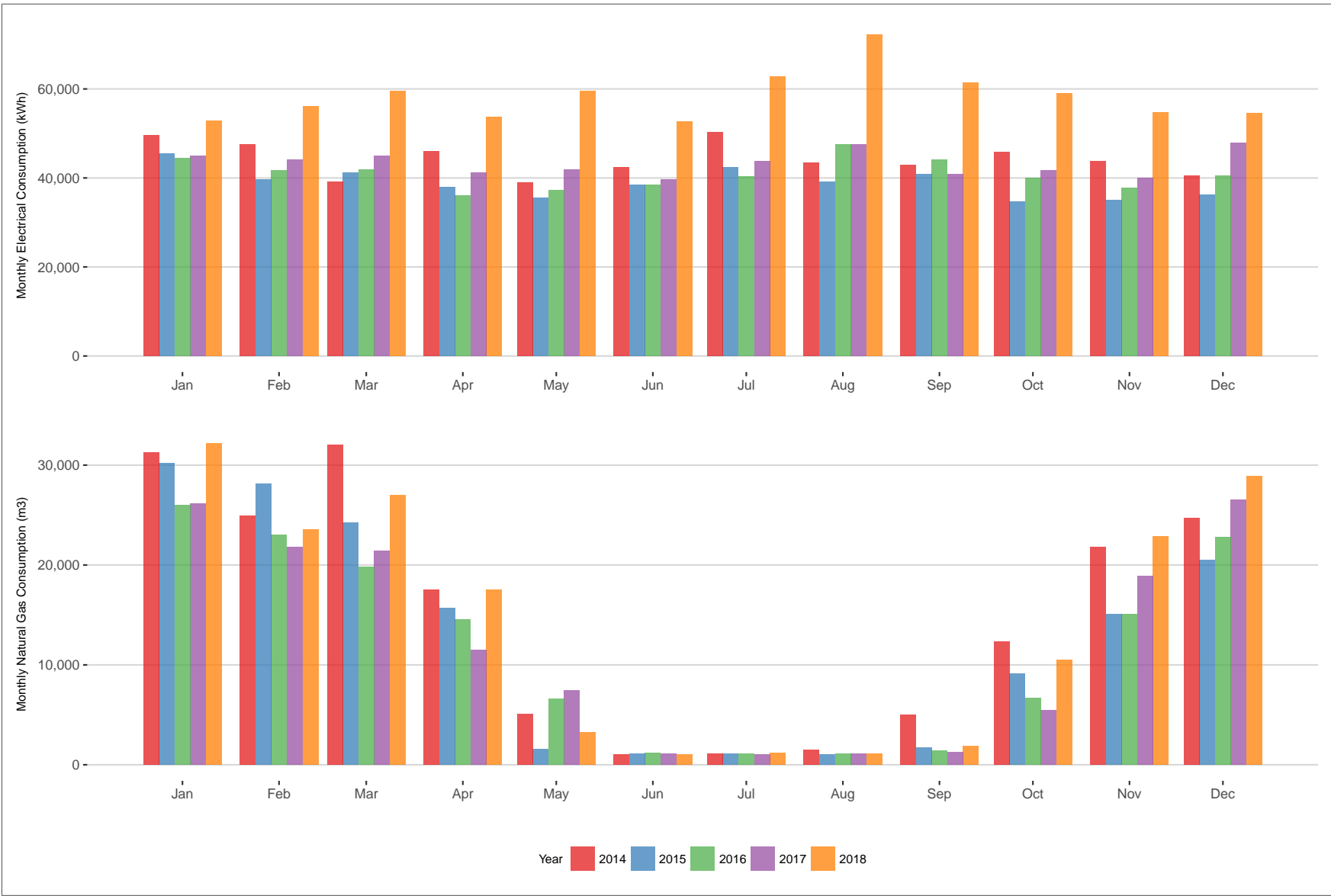
Figure 13: TWH monthly electricity and natural gas consumption
